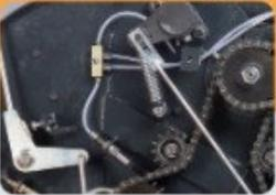
Automatic centralised lubrication system with cleaning brush
