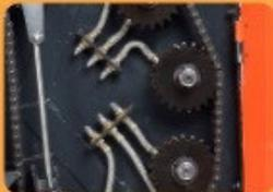
Single point greasing for Roller bearings
